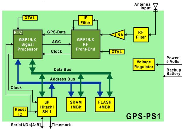
Figure 1: Blockdiagram of GPS-PS1
