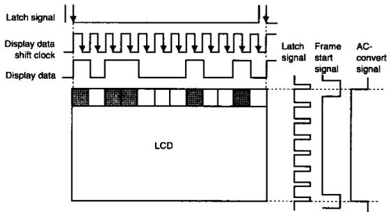
There are four display timing signals: display data shift clock, latch signal, frame start signal, and AC-convert signal.
