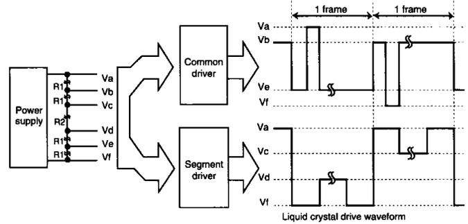
The LCD drivers are classified into two types: the common driver and the segment driver. The common driver drives common electrodes and the segment driver drives segment electrodes. As shown in the figure above, these drivers select a proper voltage level sequentially from the six voltage levels (Va to Vf) to generate liquid crystal drive waveforms. The six voltage levels are generated by resistance division.
