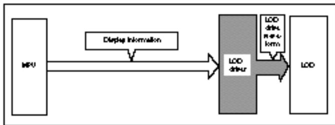
The LCD driver generates liquid crystal drive waveforms according to the display information sent from the MPU, and uses the waveforms to drive the LCD.
