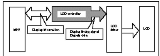
The MPU cannot directly interface the LCD driver. So the LCD controller is placed between the MPU and the LCD drivers to handle the interface between them.
