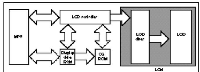
Most graphic modules feature the segment and common drivers on the LCD module, and use a 4-bit parallel interface to an external controller. The controller can be an external PC board (such as the LCDC-1330) or the controller IC can be located on the mother board with the microprocessor. In the larger graphic modules, all the board space is taken up with the driver ICs. Also for small graphic modules with high resolution, there may be no room to locate the controller on the module.
