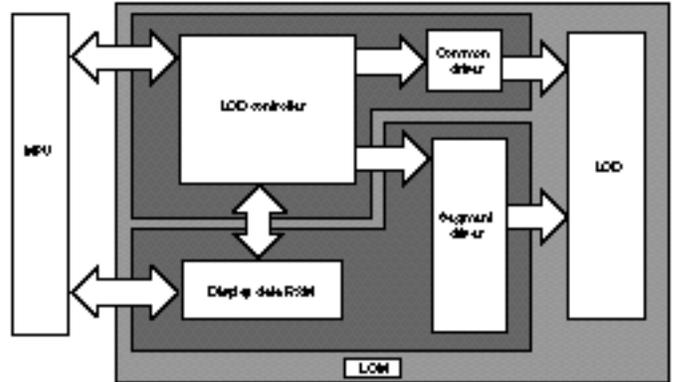
Graphic modules with built-in data RAM have two types of ICs: one integrating the controller and common driver, and one integrating the display data RAM and the segment driver. These modules use direct bitmapping; one bit in RAM corresponds to each pixel on the display. They communicate directly to the microprocessor through an 8-bit parallel interface. All the required controller timing functions are built-in to the module. There is no CG ROM, or any way to store information.
