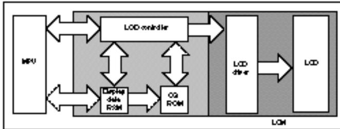
Seiko Instruments offers five graphic modules with the SED1330 controller built-in.\* These modules interface directly to the microprocessor with an 8-bit parallel interface. The 1330 was carefully chosen to offer our customers the most advanced features, including overlaid graphics and text, horizontal and vertical scrolling, built-in character generator with external RAM, etc.
