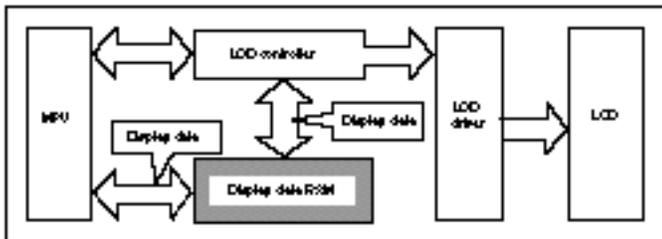
The display data RAM stores the display information sent from the MPU. The LCD controller reads data from the display data RAM, and transfers the data to the LCD drivers. Some LCD controllers let the MPU directly interface the display data RAM as shown by dotted lines in the figure above.
